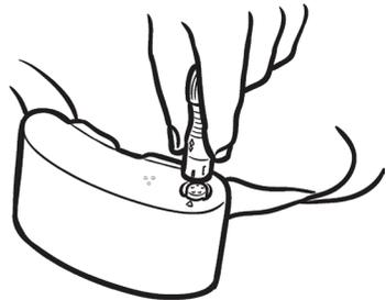
Fig. 2. Plug turbo unit power cable into battery pack
