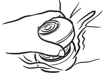
Fig. 1. Check P3 filter is fitted to turbo unit
